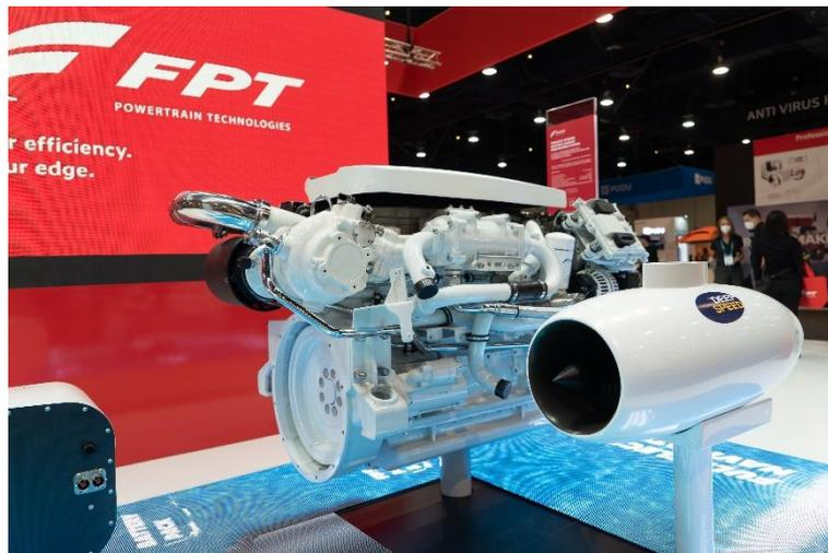
Shaped to externally resemble an aviation jet, through an integrated electric motor it sucks the water from the front and pushes it from the bow side to propel the boat. The energy for the electric motor is supplied by batteries that can be recharged on board by the **FPT Industrial N67 570 EVO engine**, coupled with a state-of-the-art variable generator, or by the charging station when the boat is in harbor mode.
